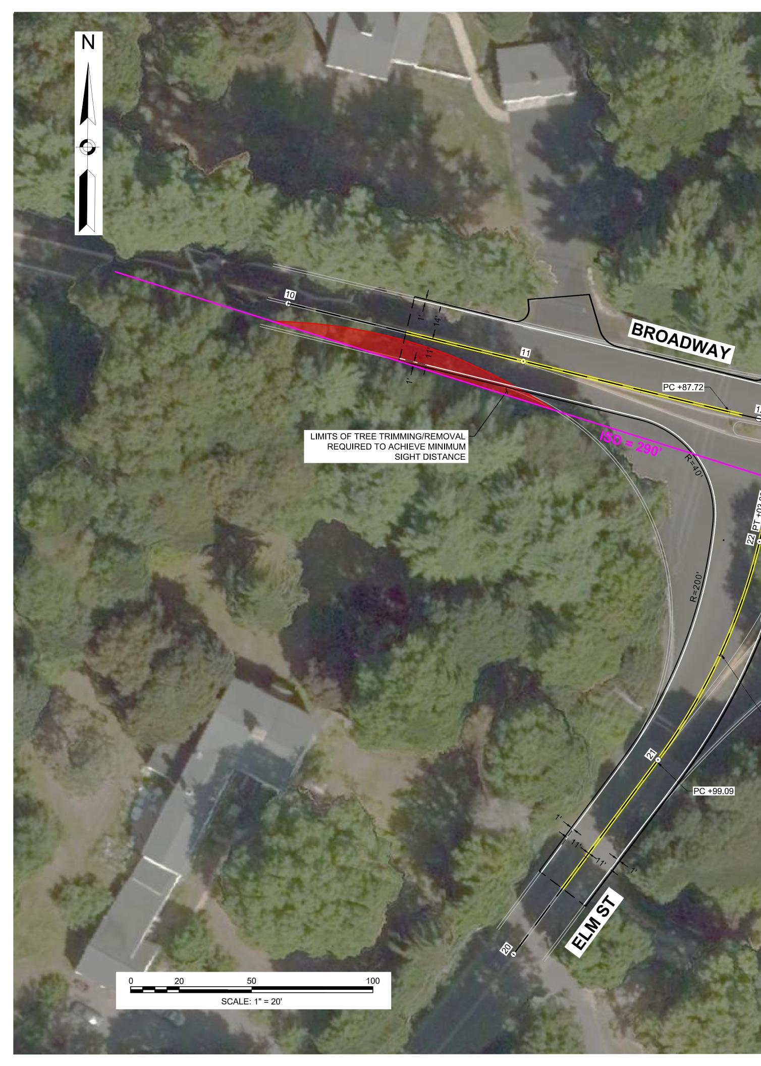
LIMITS OF TREE TRIMMING/REMOVAL REQUIRED TO ACHIEVE MINIMUM SIGHT DISTANCE
