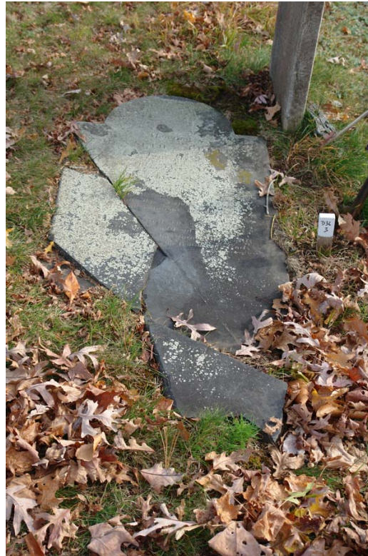
D.36.3 Seth Curtis— as found, requiring structural adhesion
