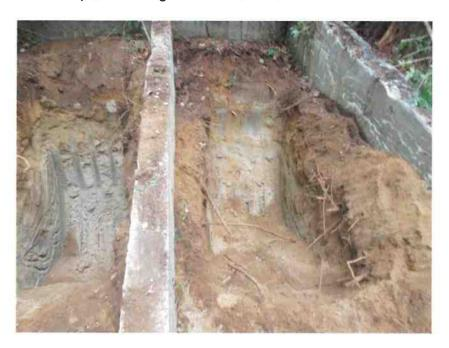
**4.)** Excavation test pits foundation # 2 (southeast) eight (8) feet below grade, sand and gravel and silty / clay soils. No debris, no olfactory odors, no stains, no PID readings. Note: sampled for magnesium and 8 RCRA metals.
