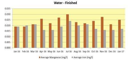
Finished Water quality remains strong at all three treatment plants with iron and manganese levels well within our treatment goals. This is further evidenced by the relative lack of water quality complaints which we believe is a function of finished water quality and the effectiveness of the spring and fall flushing programs.
