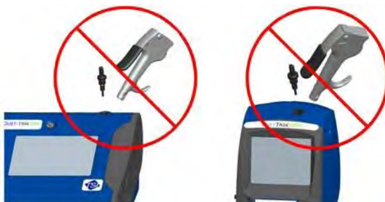
Figure 4-3: Do NOT Blow into Instrument
