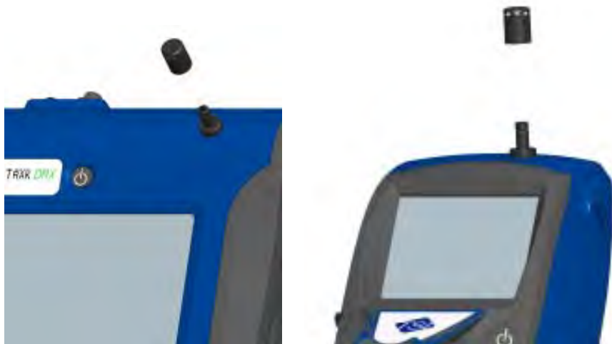
Figure 2-6: Putting on Inlet Cap
