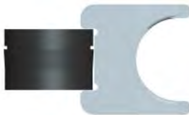
Figure 4-20: Replace Mesh in Filter Holder
