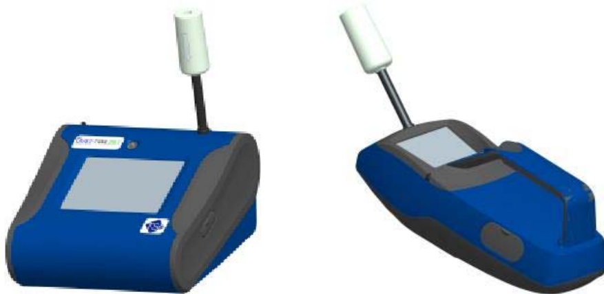
Figure 4-1: Attach Zero Filter to Inlet
