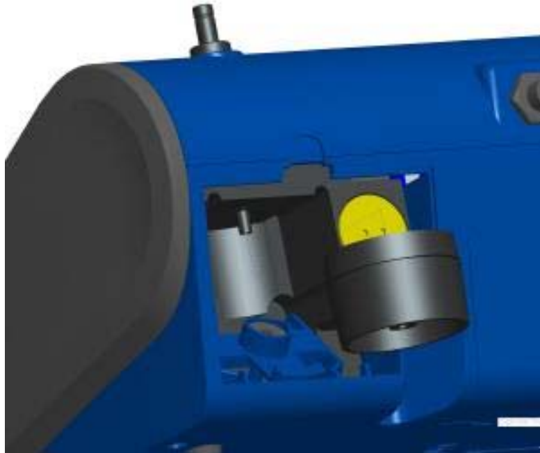
Figure 4-8: Remove 37-mm Filter Cassette
