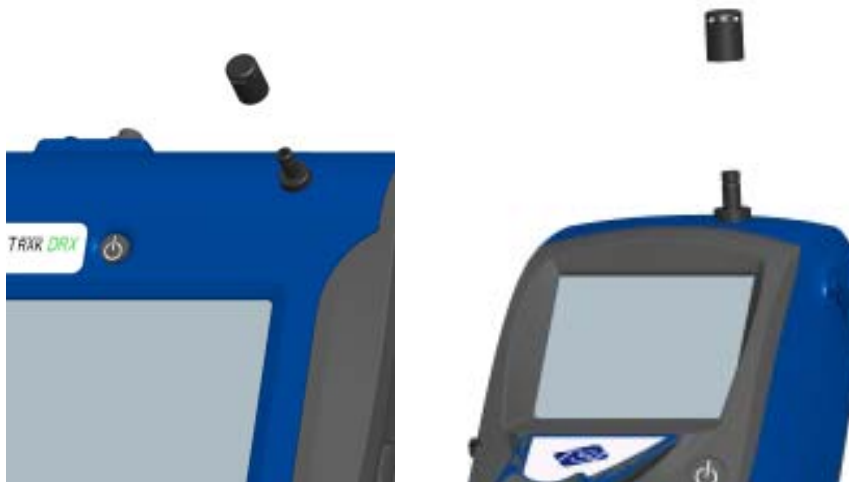
Figure 2-6: Putting on Inlet Cap
