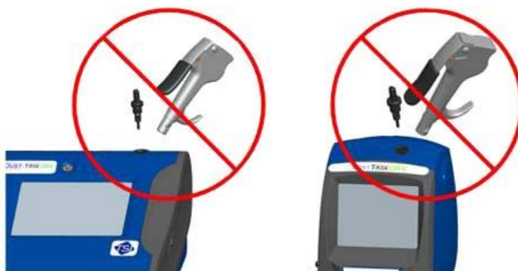
Figure 4-3: Do NOT Blow into Instrument
