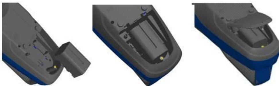
Figure 2-2: Batteries into Handheld Unit
