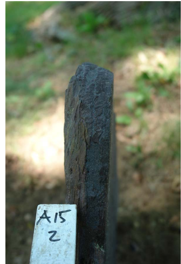
#A15.2, Jemima Farrow. Before and After. Delaminations filled with Sto Crack Filler
