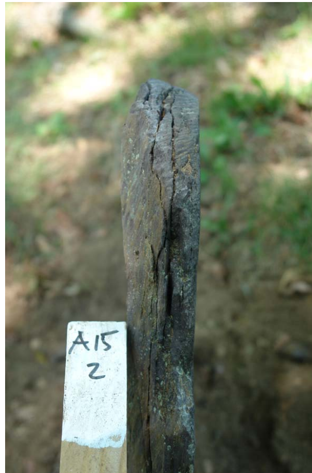
#A15.2, Jemima Farrow. Before and After. Delaminations filled with Sto Crack Filler
